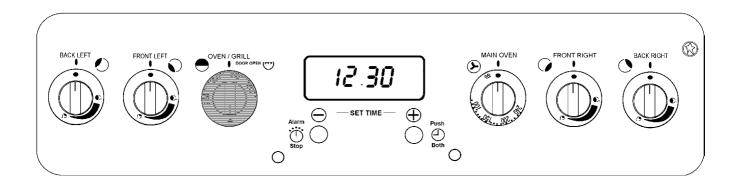
To operate the top oven turn the temperature control to the required setting. Our diagram shows the oven set to 160°C. Close the oven door.
